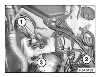
Detach pipe (1) from intermediate piece (2) and from master brake cylinder (3). Remove pipe with rubber grommet.**Installation**:
