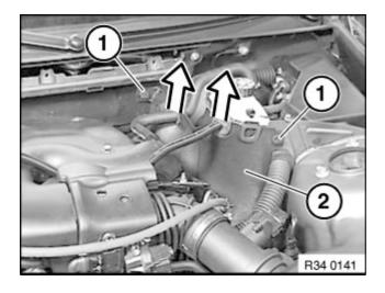
Remove vacuum line and B+line from assembly compartment partition wall.
