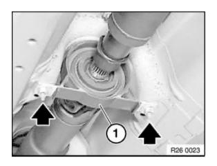
Grip propeller shaft and release nuts.
