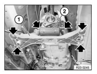
Release screws and remove cross-member (1). Tightening torque 23 71 1AZ / 2AZ .
