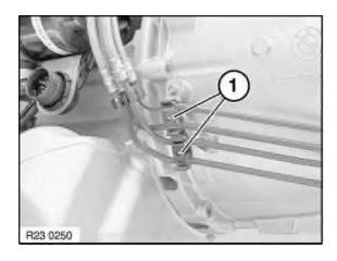
Unclip hydraulic lines at holders (1).
