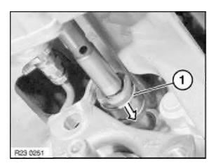
Lever out retaining ring (1) with a screwdriver. Push retaining ring (1) forwards slightly.
