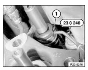
Drive out retaining pin (1) on selector rod linkage with special tool 23 0 240 .
