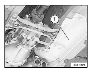
Remove heat shield (1). Remove holder for engine underbody protection at rear.
