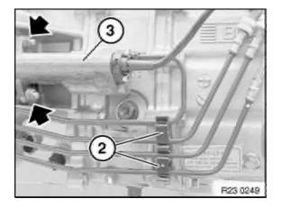
Unclip hydraulic lines at holders (2).
