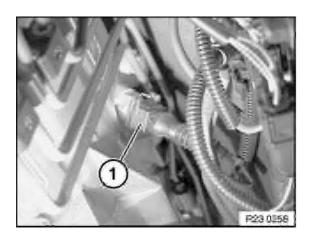
Disconnect plug for reversing light switch (1).
