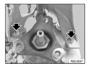
Release screws on actuator.
