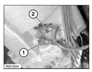
Disconnect plug for transmission oil temperature sensor (1) and transmission speed sensor (2).
