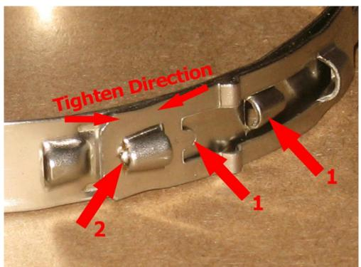
The quick install hose clamp has two lock positions. The first lock position is engaged when tab (1) is inserted into opening(1) indicated by arrows (1). In this state the ring is locked but is not tightened. The second lock position is labeled by arrow #2, when a small sharp tab is inserted into a smaller opening.
