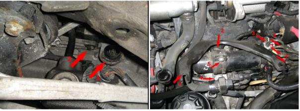
Secure smg pump from underneath a car with bolt (2) as well as from the top bolt (4). Loosen up bolt 5 so that smg pump can move freely inside the brace.
