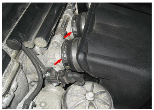
Remove six quick release hose clamps connecting air-box cover to throttle bodies. (In order to make your job easier a special bmw tool should be used to perform this procedure. Unfortunately, because of the cost, I used needle nose pliers, which made the job more difficult)
