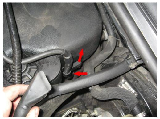
• Detach wire by sliding up support clamp
