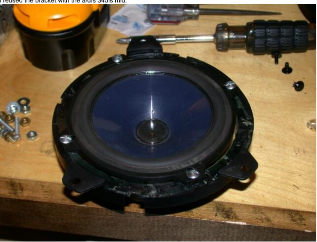
and since it was a little bit smaller I used some 3/8" thick foam I had to create a ring to seal the new "smaller" speaker to the door panel:
