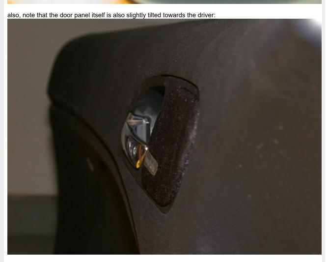
Not that you need to know this for this upgrade, but the only way to get the mesh out of the door panel is to remove the door panel and remove the tweeter/mid. It is just clipped in place:
