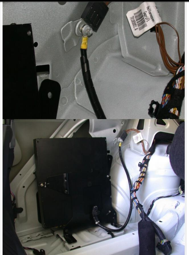
Of course, use heavy gage wire with an in-line fuse as close to the 12+ terminal as possible (notice I used cable ties everywhere – no room for accidents!):
