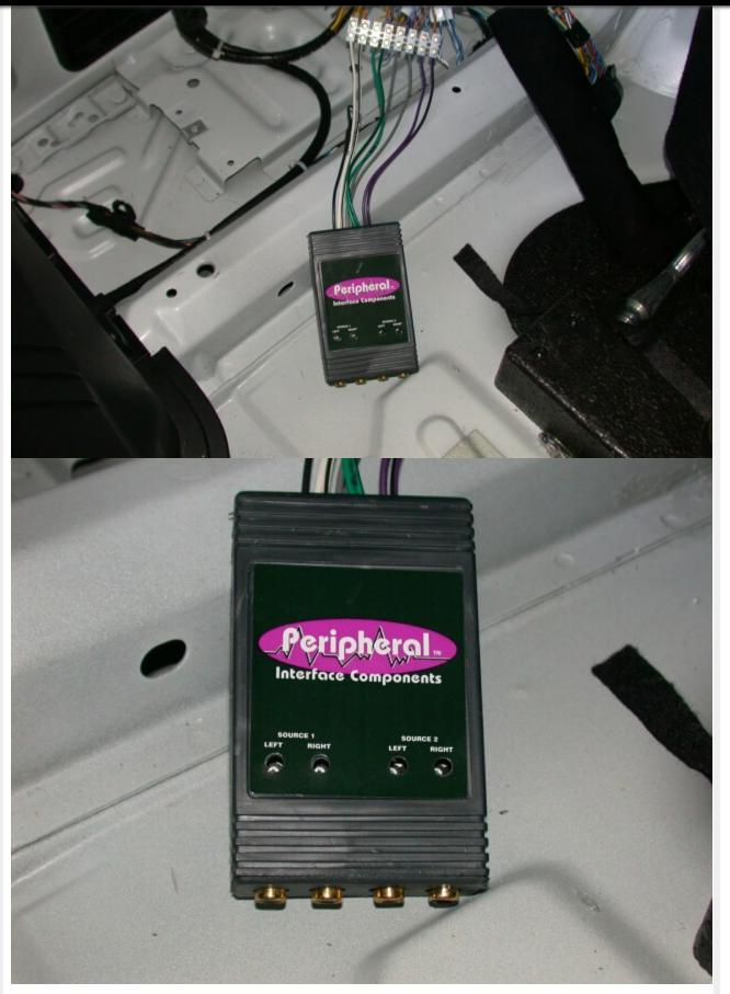
You probably noticed that I am using screw-type white posts to get signals together. Not only these are electrically strong, but allow me to re-wire as appropriate (which I did since I first wired the amp to the stock speakers, and then later to the external passive crossovers for the separate front components). Pick the right method to fit your needs.
