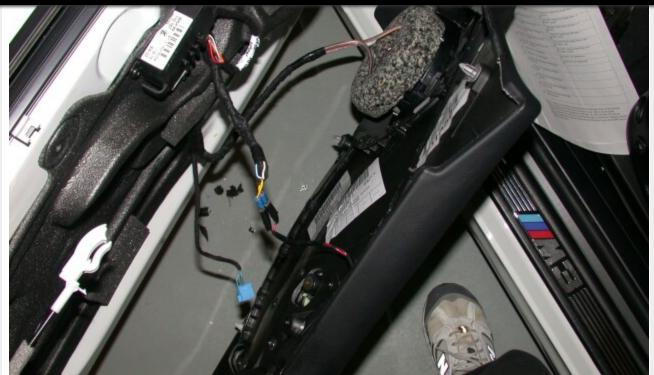
I did the right door next, and then went back to finish the amplifier/crossover installation. I did try the front speakers with the a/d/s amp but without their a/d/s speaker crossover units and the new a/d/s speakers did not sounded good at all — I simply could not adjust the level and frequency balance to match the carefully developed a/d/s crossover, but at least I was able to verify that the speakers were wired properly.
