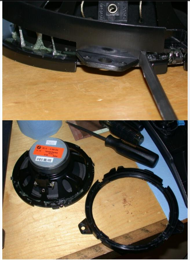
And removed the ring which remains on the door panel, which is not being reused:
