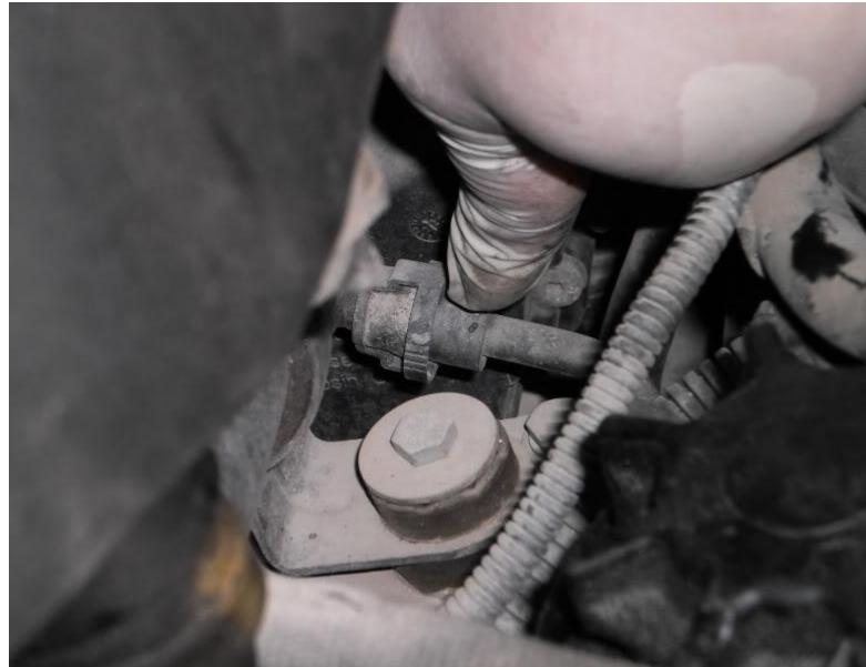
2d. DO NOT go and buy the special tool for removal of the clamps. If you go into the trunk of your car and get the wrench out you can remove them with that. I suggest compressing to 2 sections furthest away from the end of the clamp and pull backward.
