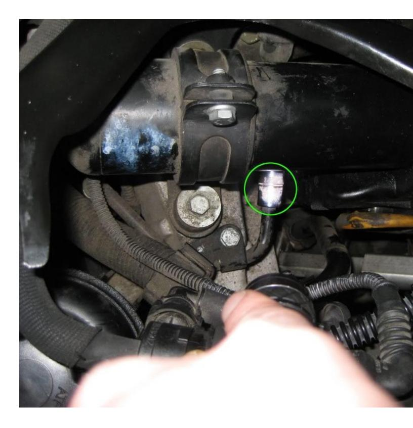
15. Once that is done insert the airbox into the rubber air tubes and position the grommet/bolts into the airbox bracket. Then bolt on the 10mm bolts until they are lightly snug. Once that is done reattach the bottom forward hose and the two top hoses.
