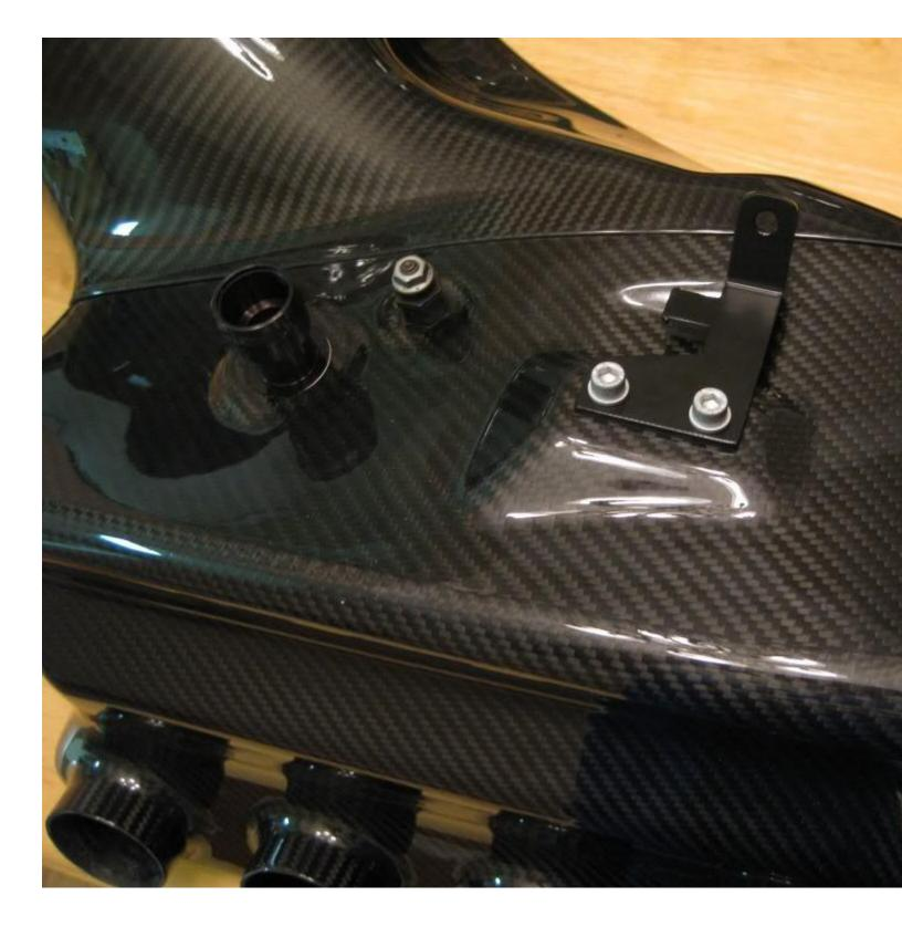
6. Find the OEM intake and flip it upside. You'll want to remove the grommet/bolt pieces and install them on the new airbox. A 15mm wrench will remove these. I cleaned mine up before installing them on the new airbox. The grommet/bolt I'm referring to is #4 in the picture below.
