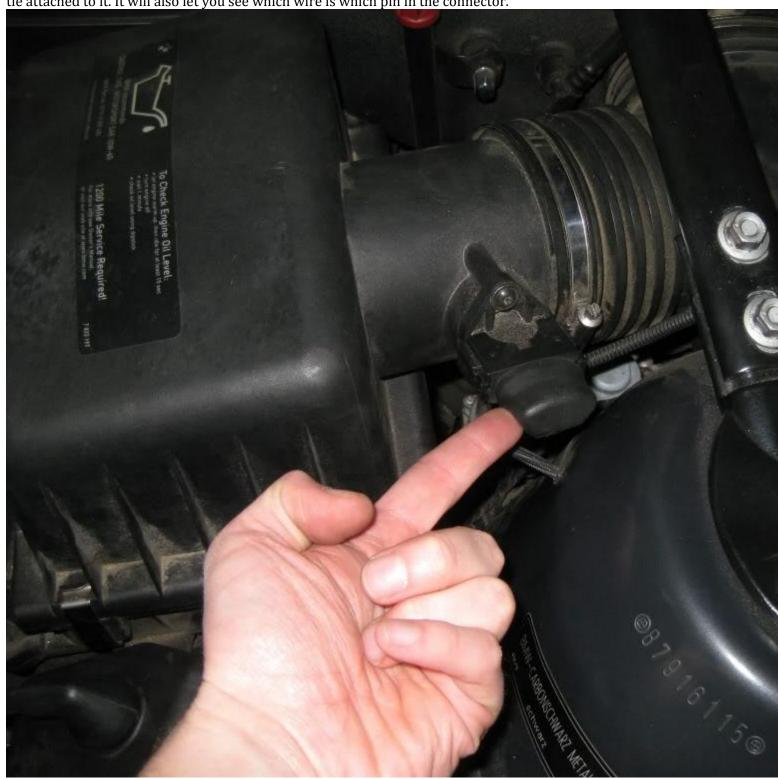
Here is the MAF connector without the rubber grommet around it. You can see where pins 1 (Blue/Yellow) and 3
