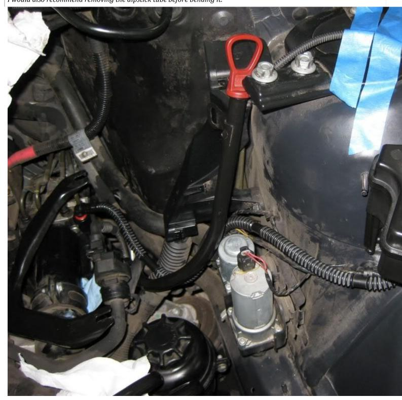
14. Now it's time to install the first half of the CF airbox. Begin by rerouting and reconnecting the oil bypass valve. It will be the most annoying thing to reinstall outside of the rear 10mm bolt that connects to the airbox bracket.
