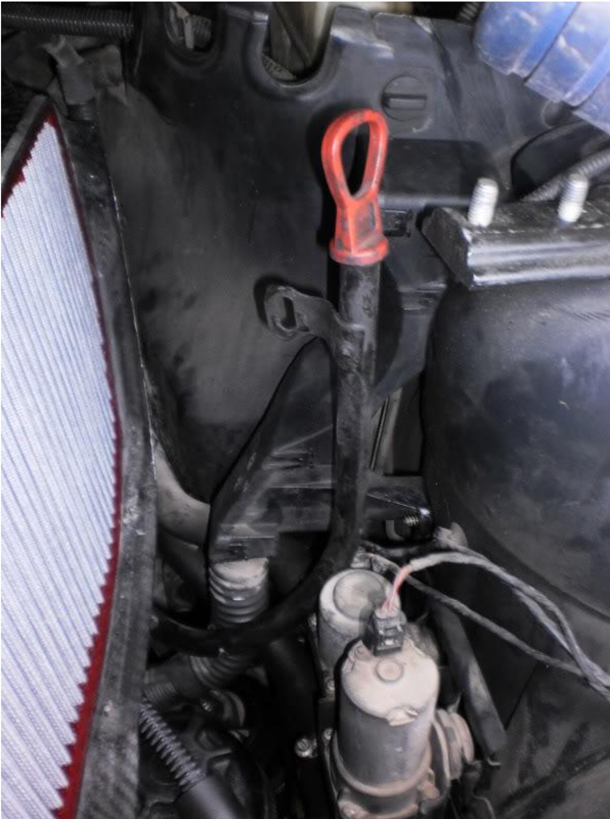
Plug in the OEM CSL SMG fluid reservoir. this picture shows the bracket of the smg tank on an OEM CSL that happen to be in the garage at the time
