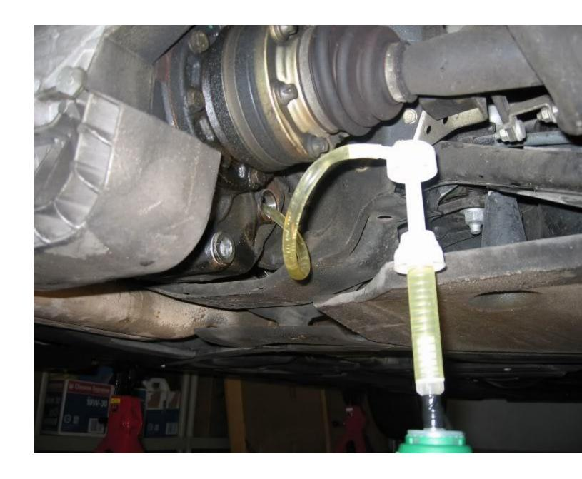
7. Put fill bolt on with washer and tighten it to 48 ft-lb. I had hard time fitting torque wrench for fill bolt, so I had to use combination of some adjustments shown below.
