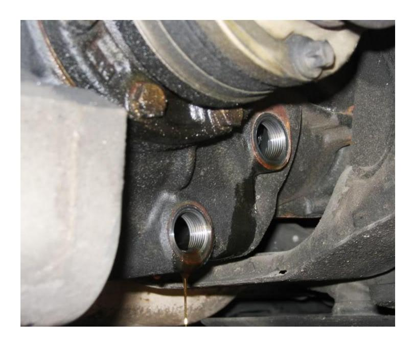
5. After complete drain of the old fluid, put drain bolt back on. I noticed that drain/fill bolt has green rubber o-ring on them, but since I bought washer, I put them on and tightened to 48 ft-lb. According to Bentley service manual, torque spec for drain/fill bolts are:
