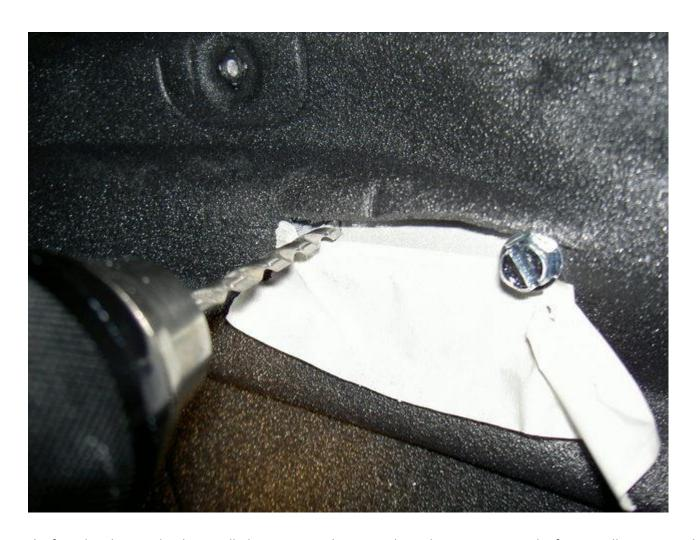
the front bracket need to be installed in a near 45 degree angle as shown - cut away the foam to allow proper placement. if you chose to use the sheet metal screw and self locking washer, don't gorilla the sheet metal screw - it will strip the thin door metal. just get it tight enough that the self locking washer flattens - it will not come loose
