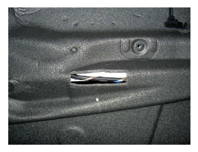
i use a drill bit that is slightly smaller than the sheet metal screw and tape up the lower portion of the foam opening to prevent loose sheet metals from falling inside of the foam/door while drilling - they can rust and stain the door
