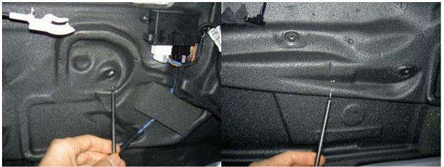
place the bracket on the door panel so the wite-out marking placed earlier can be seen through the center opening and mark the location of the anchor screws. now carefully cut away the foam to make room for the brackets. the rear bracket location has a wire bundle under the foam. take care not to cut the wire or gouge the paint.
