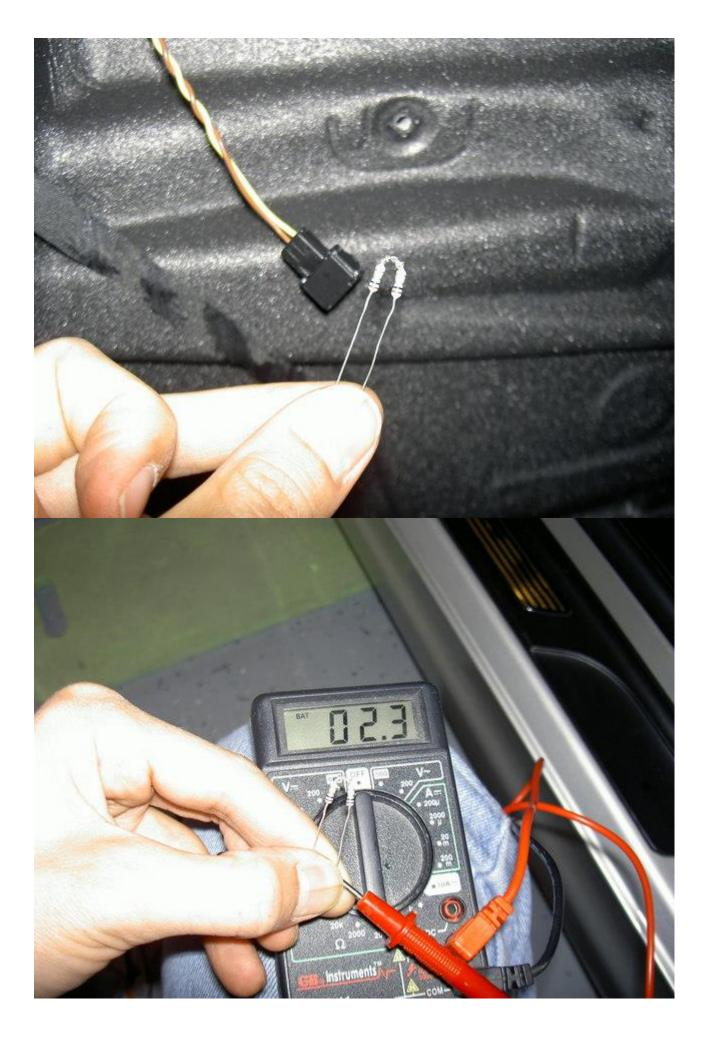
place it in the side air bag connector and wrap the resistor with electrical tape. tape it to the foam on the door and you are done  $\dots$  ready to install door panels
