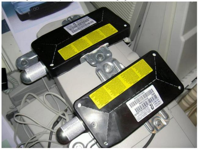
to fool the car that the side airbags are still connected - you need to insert some form of resistor rage 1.5-2.5 ohms. i use two 1/4 watt 1 ohm connected in series to make it approx 2.3 ohms (they have 5% variance in resistance). these resistor can be had from Frys electronics or any local electronic stores. don't measure the resistence on the airbag directly. you may set it off lol
