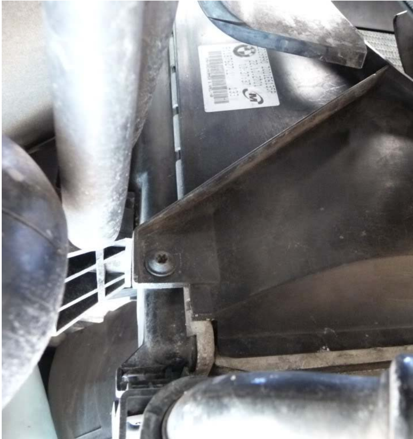
The oil cooler is also held on by four bolts, two per side
