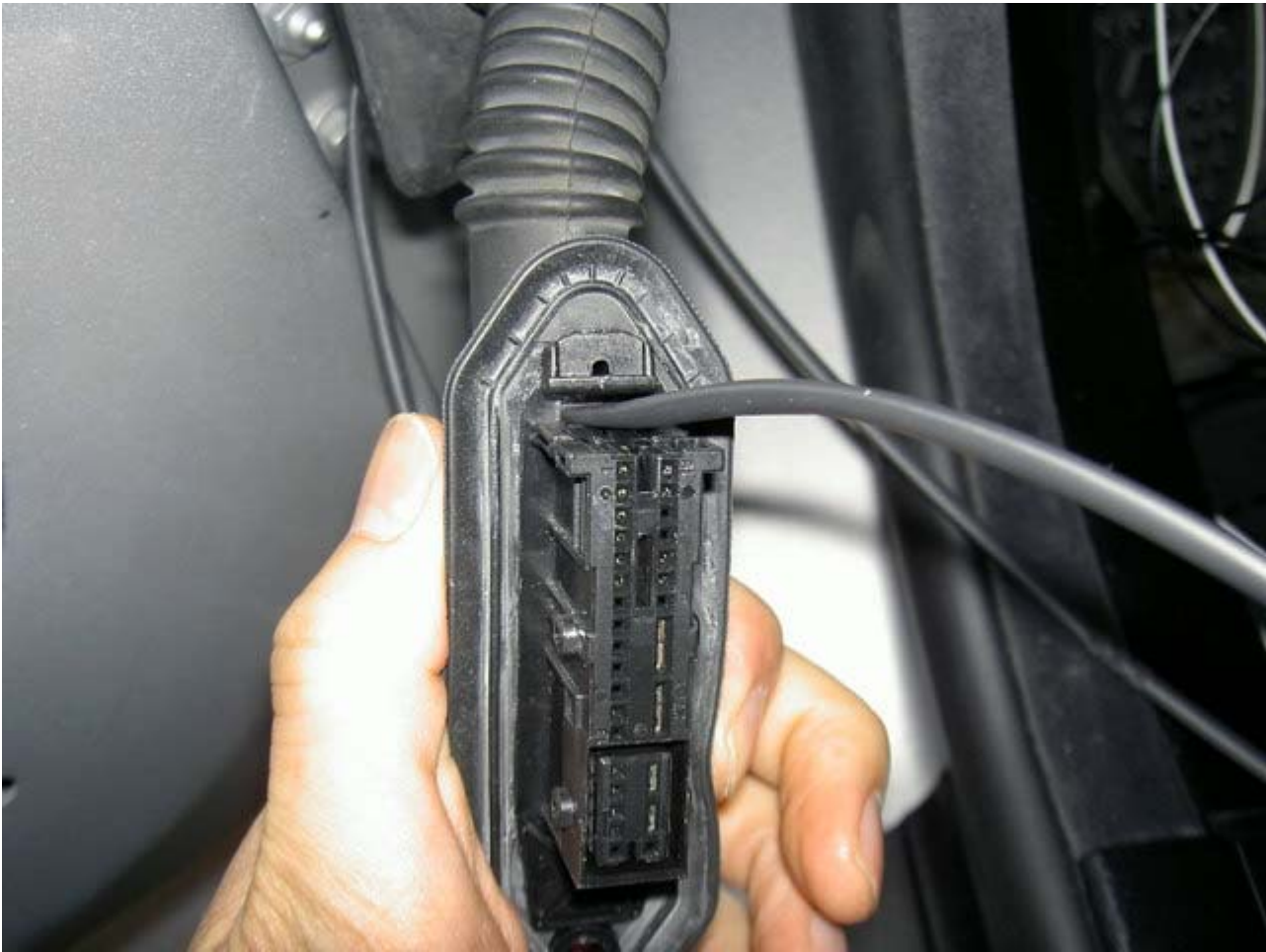
the routed wire will sit nicely on the lower end of the wire harness
