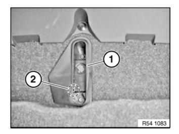
Remove convertible top compartment floor from centre mount (1).*Installation:*Insert convertible top compartment floor from above (above microswitch 2) into centre mount and
