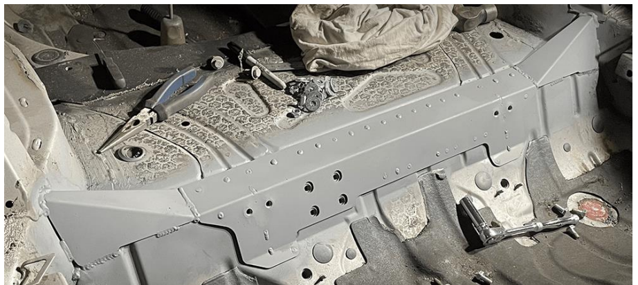
Figure 28 – Installed CMP front RACP reinforcement kit
