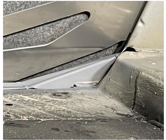
Figure 27 – Rear stitch weld location.
