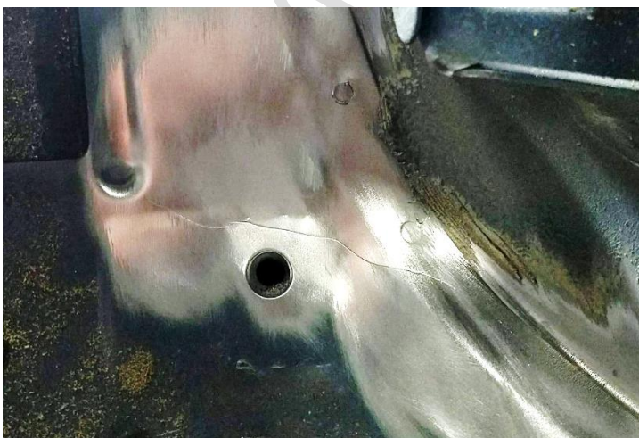
Figure 6 – Crack above far left anchor point.
