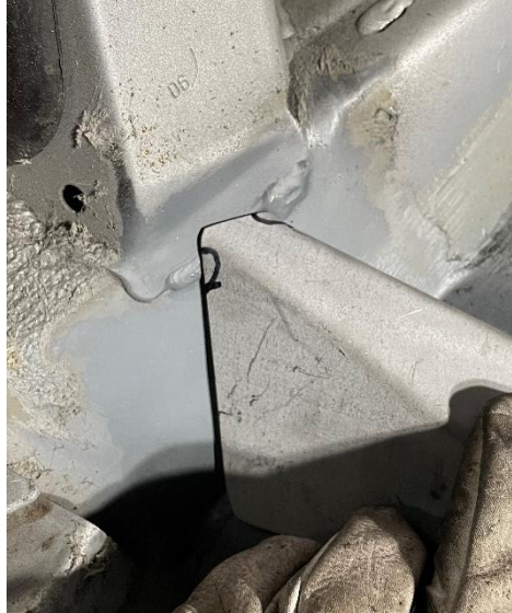
Figure 24 – bulkhead weld marked on chassis gusset.
