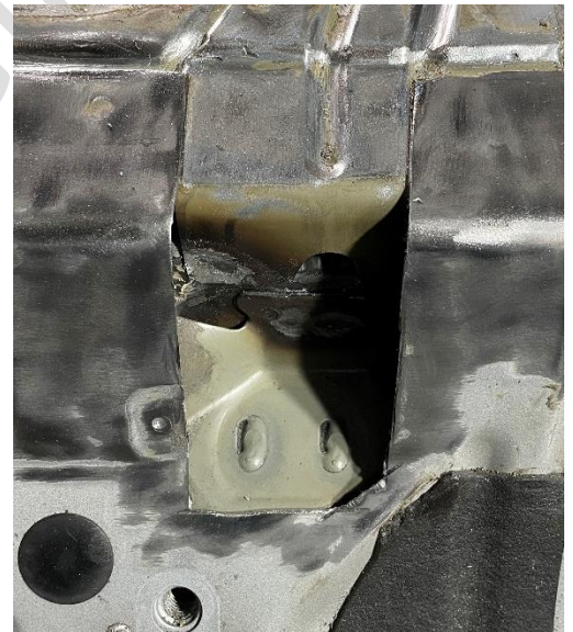
Figure 3 – Front subframe mount top welds.
