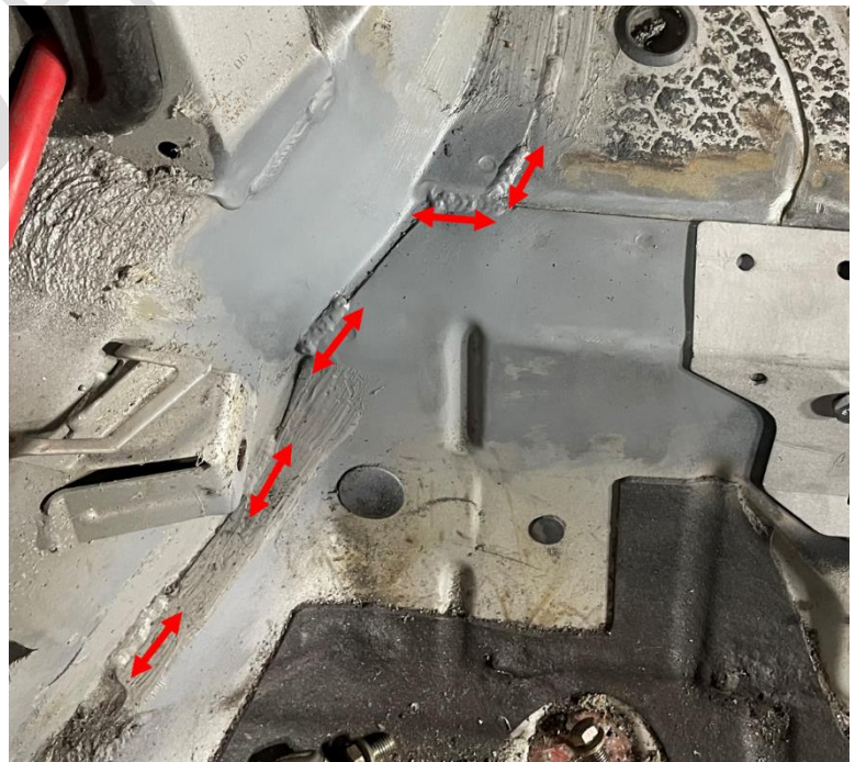
Figure 11 – Bench seat panel to chassis rail stitch weld locations.
