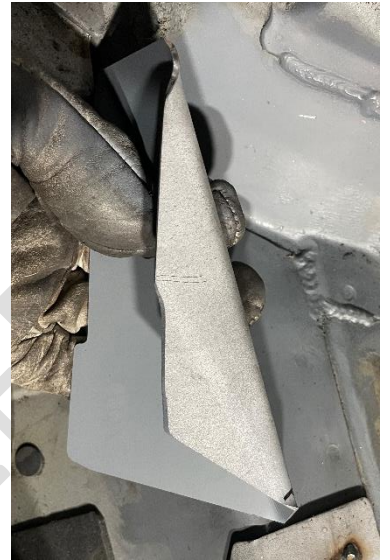
Figure 25 – Chassis gusset clearance for stitch weld.
