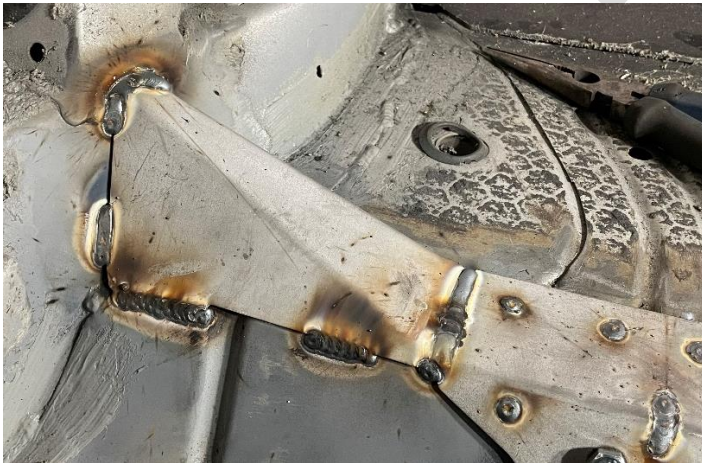
Figure 26 – Chassis gusset front weld locations
