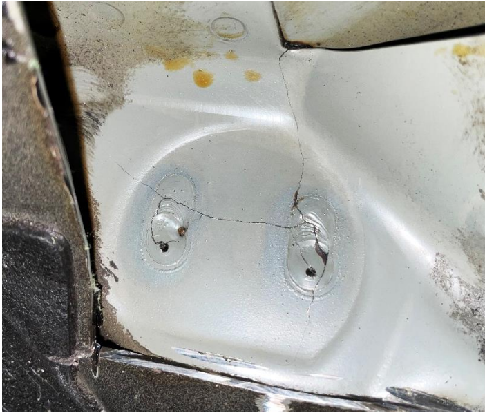
Figure 4 – FR top weld cracks.
