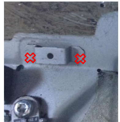
Figure 1 – Bracket spot welds location.
