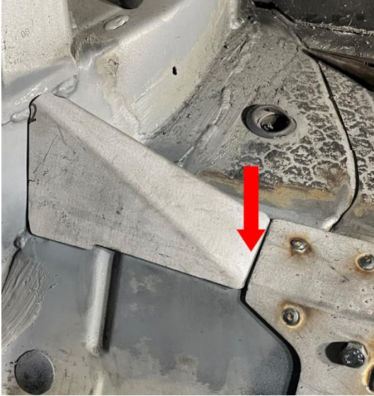
Figure 23 – Push chassis gusset down here.
