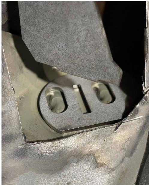
Figure 13 – Mount gusset locating notch.
