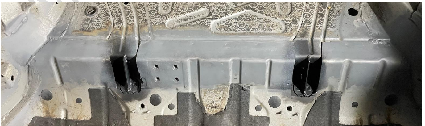
Figure 19 – Primed front mount topside ready for bar install.
