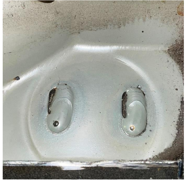
Figure 5 – FL top welds cracks.
