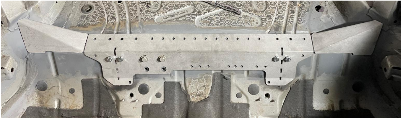
Figure 2 – Front RACP reinforcement kit test fit.
