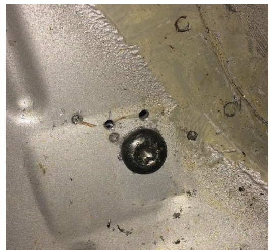
Figure 7 – Anchor point crack stop drilled.
