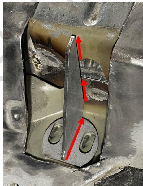
Figure 18 – Mount gusset weld locations.
