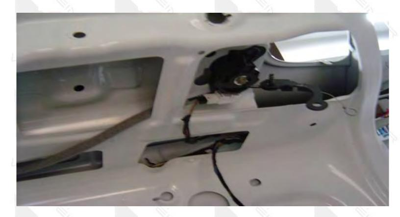
Rap some tape around the ends of the plugs of the wire loom. This will make it easy to pull the wire loom out of the trunk. At this time also remove all other components in the trunk.
