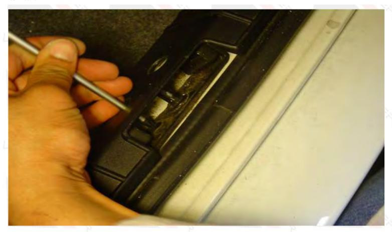
You can adjust the trunk to move left or right by adjust the 4 torx screws on the hinges. Do so by apply some horizontal force and slowly push the trunk the direct you want to move.
