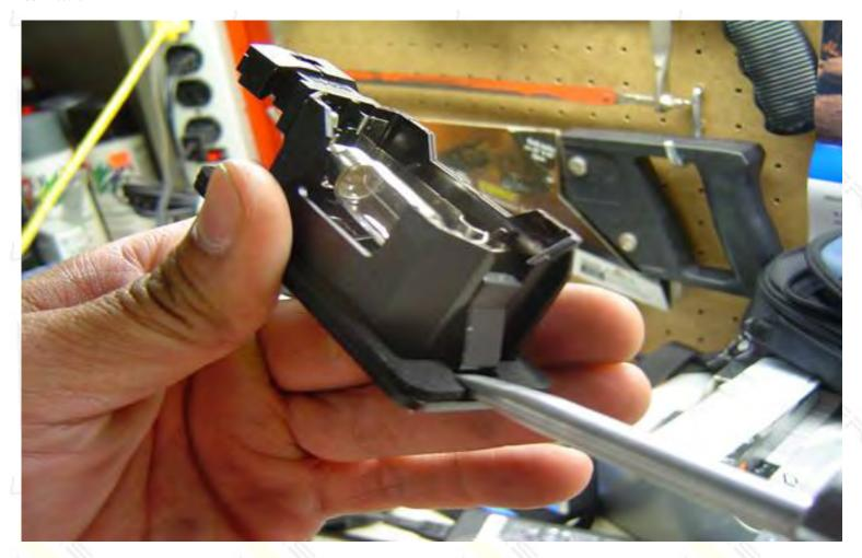
Here is the other side of the light. This is the area which latches to the trunk.
