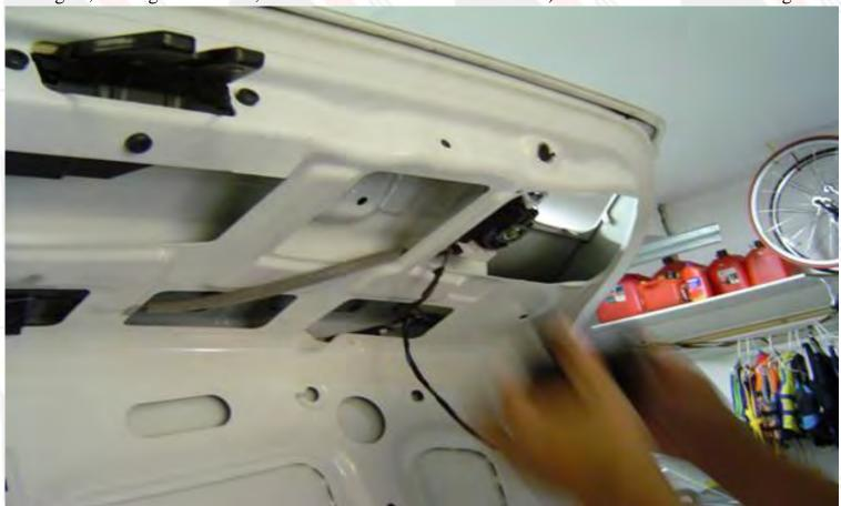
Remove the locking mechanism. Pull the center out first, you can use a flat head screwdriver to pry it apart. Then remove the 2 torx screws. The locking mechanism comes out by turning it clockwise.
