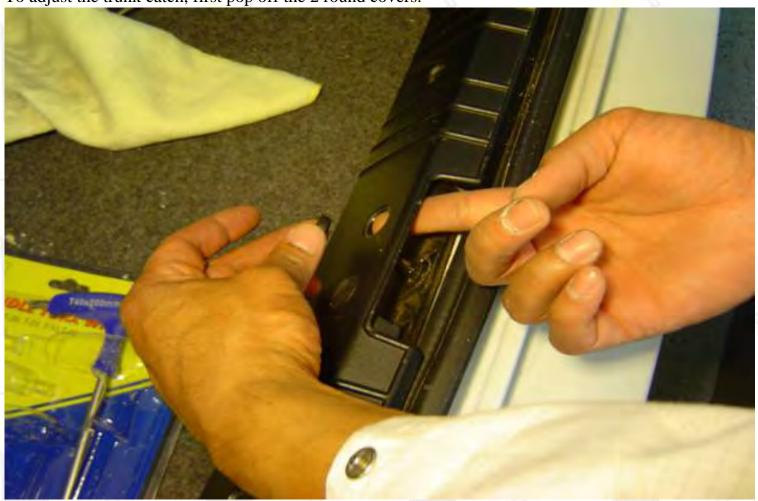
Adjust the trunk latch about ¼". Some trunks may need more or less adjustment. Adjust the catch so the striker from the trunk latch is centered correctly.
