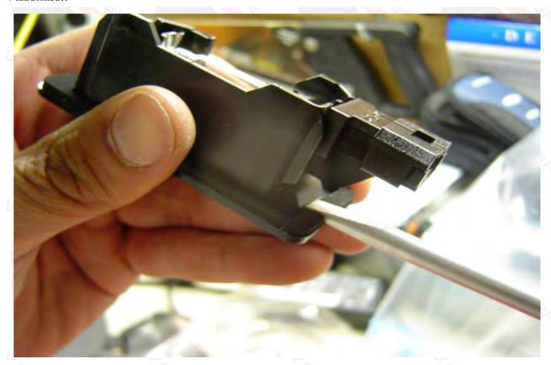
Push the light up and slide it over with a screw driver until it catches.
