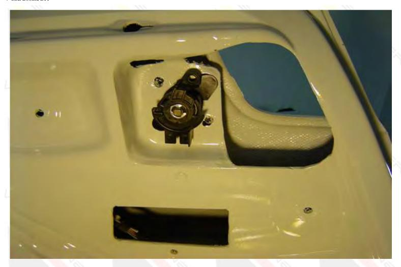
Re-install the trunk latch. Also re-attach the plugs for the locking mechanism and trunk latch.
