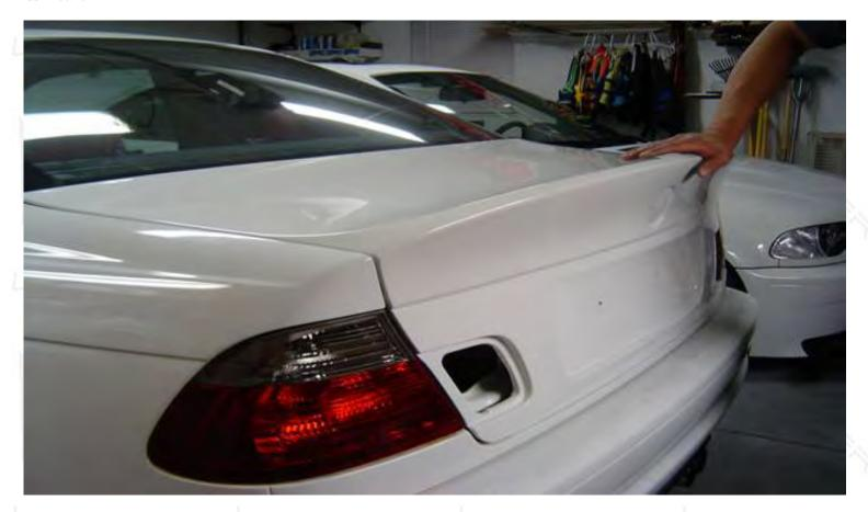
Let's first re-install the locking mechanism. Place the rubber grommets on the outside of the key opening and install the locking mechanism counter clockwise. If the torx screw holes don't line up properly, simply dremel the holes bigger.
