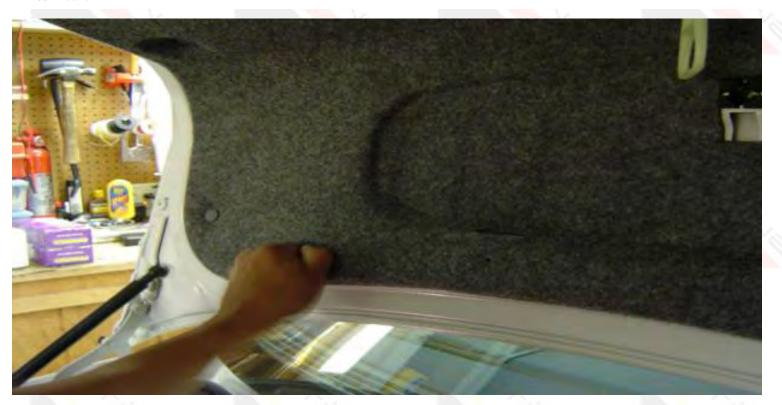
Unplug all the connectors from the wire loom. There should be 5 total connectors to remove. (plugs -2 reverse lights, locking mechanism, trunk release button and trunk latch). Now remove the reverse lights.
