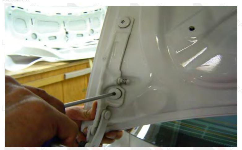
Repeated adjustments to these 4 torx screws may be required in order to have your bootlid centered onto the car. Remember to apply constant pressure with your thumb to move the trunk in the direction you want as you loosen and tight the 4 torx screws.
