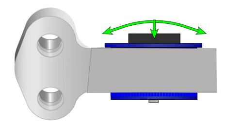
o If the spherical bearing is binding after installation, press it back out, thoroughly clean all burrs from the OD of the bushing and bushing bore in the lollipop housing, then press the bushing back into place. In some cases, you may have to do this more than once, depending on variations in the tolerance of the bracket bore.
