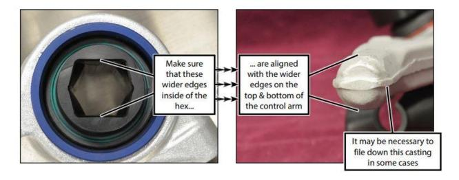
If the hex is correctly oriented and the issue still persists, the hex transition of the control arm may need to be filed/ground to allow the insert to be installed further.
