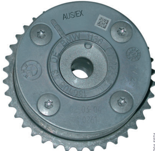
27 - Front view of VANOS unit for exhaust camshaft
