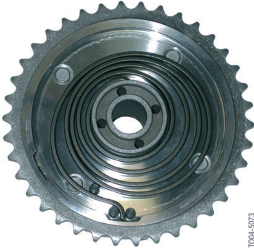
26 - Rear view of VANOS unit with cover removed
