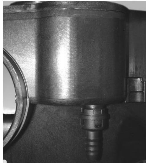
Hydraulic Fluid Expansion Tank Quick Release Coupling.
