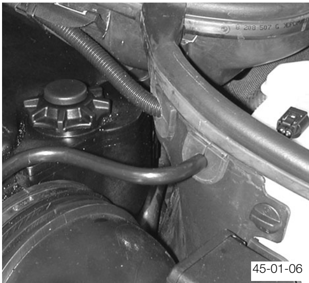
Hydraulic Fluid Expansion Tank Mounting
