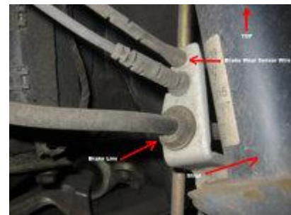
Brake Line/Wear Sensor Wire Retaining Bracket
