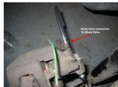
Drain Hose Attached To Valve (from above caliper)
