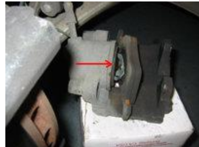
Releasing the Inboard Pad
