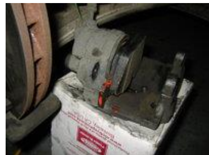
New Inboard Pad in Caliper
