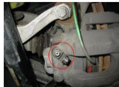
Valve Exposed (from rear of caliper)
