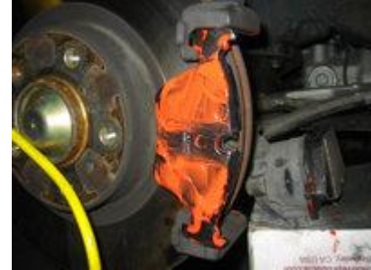
New Outboard Pad in Carrier
