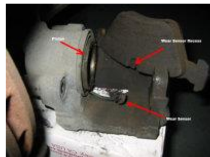
Brake Wear Sensor
