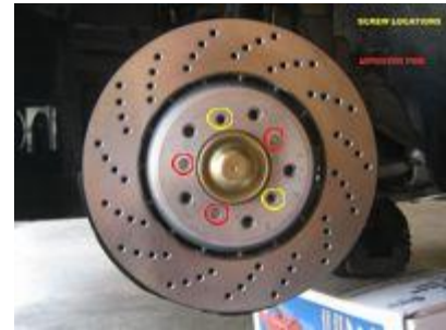
New Rotor on Hub
