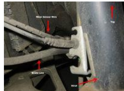
Line/Sensor Wire Released From Retaining Bracket
