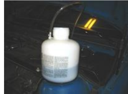
Filling the Pressure Bleeder
