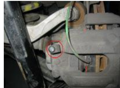
Rubber Bleed Valve Cap (from rear of caliper)
