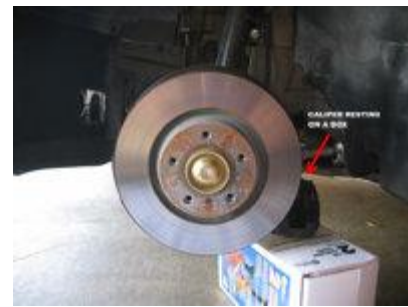
Removed Caliper "Resting"
