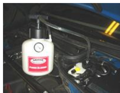
Testing the Pressure Bleeder
