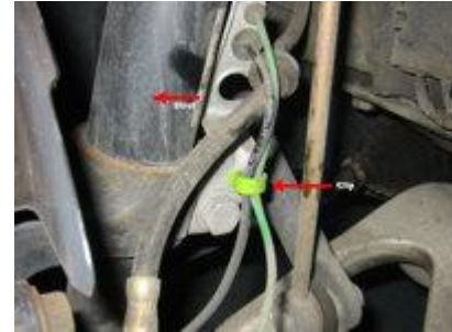
Retaining Clip (view from behind the strut)
