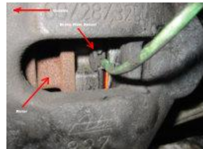
Brake Wear Sensor
