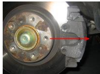
Pulling Caliper Off
