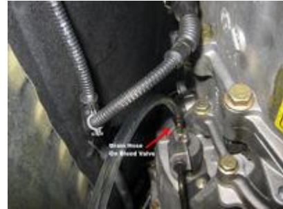
Drain Hose on Valve
