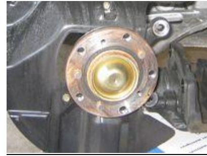
Hub with the Rotor Off
