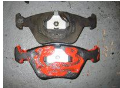
Inboard Pads Old Pad, top New Pad, bottom
