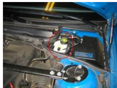
Brake Fluid Reservoir Location
