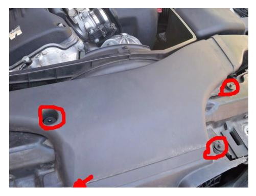
5. Remove the engine air filter box by first popping off the cover for the xenon stuff right next to the
