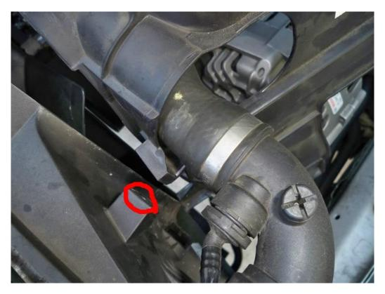
7. Pull the plug at the top of the clutch fan shroud on the passenger side. Using a T-25 torx remove the 2 screws that hold the top of the fan clutch cover in place then remove then go under the car to remove the ones at the bottom of the cover (pictures of these not shown).
