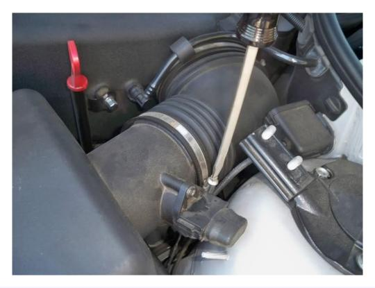
6. Remove the plastic shields that are held in place by more pins. Using a small flathead makes these easier to pop out. Remember to pop the "head" of them out before trying to pull the base. The shield on the driver side will simply rest on the coolant hose since it can't be removed completely.
