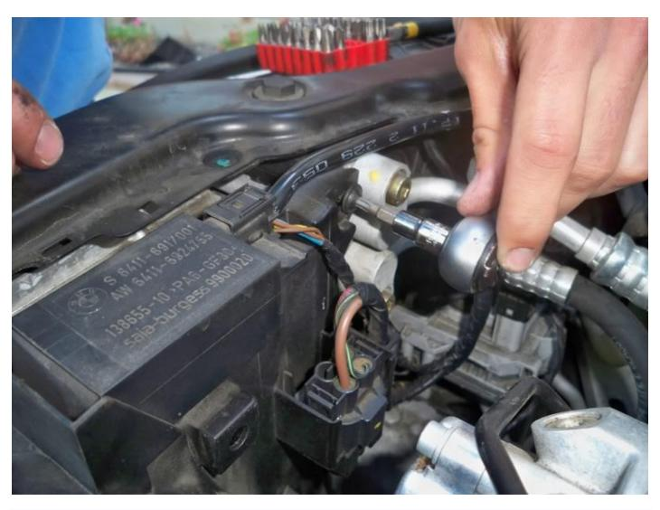
8. Remove the cabin filter housing by first removing the top piece and the filter underneath. Using a T-30 torx (going off memory so correct me if I'm wrong), remove the 4 screws and and pull the cabin air filter housing out.
