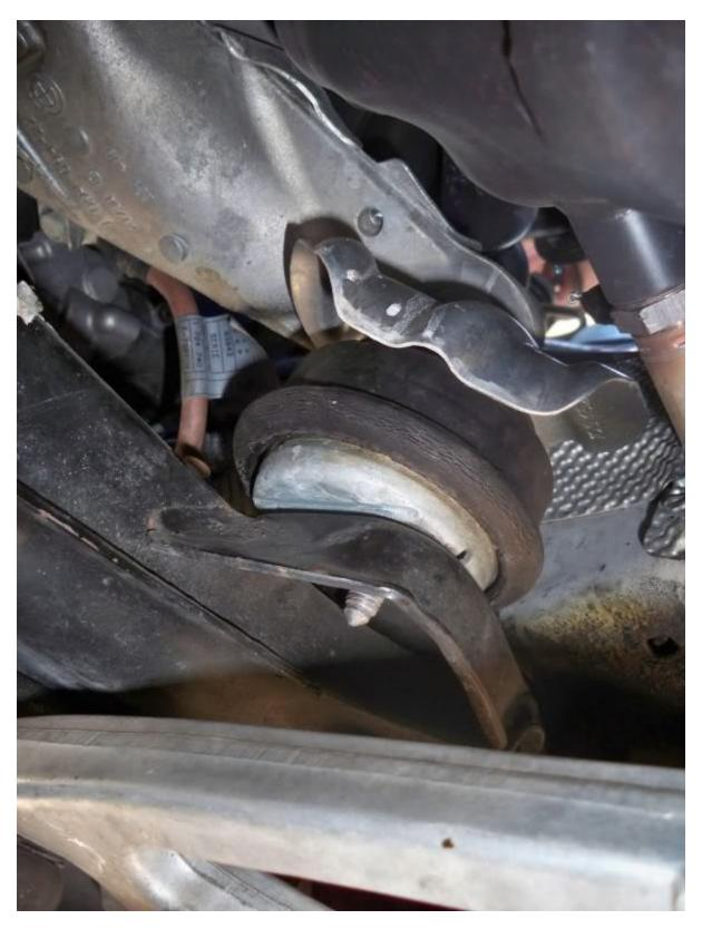
10. Remove the top nut of the passenger engine mount using a series of extensions, a universal joint, and a 16mm socket and then go under the car and remove the bottom nut. Place a 2x4 on top of a jack and
