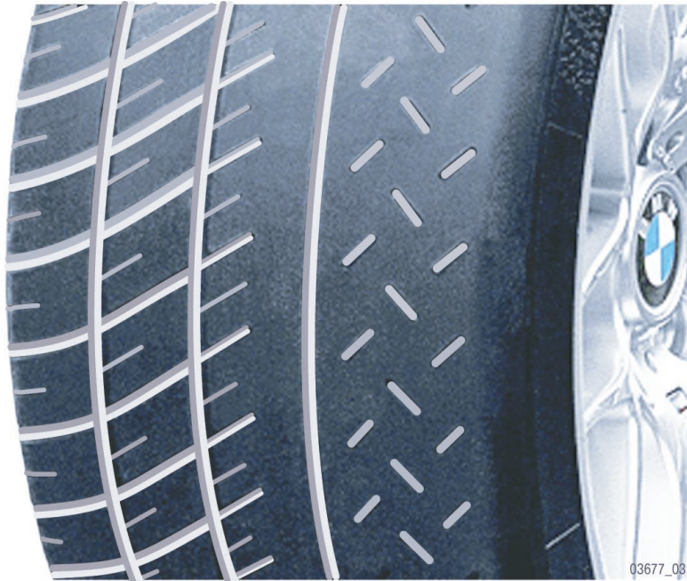
Fig. 32: Tread pattern of Cup tyre
