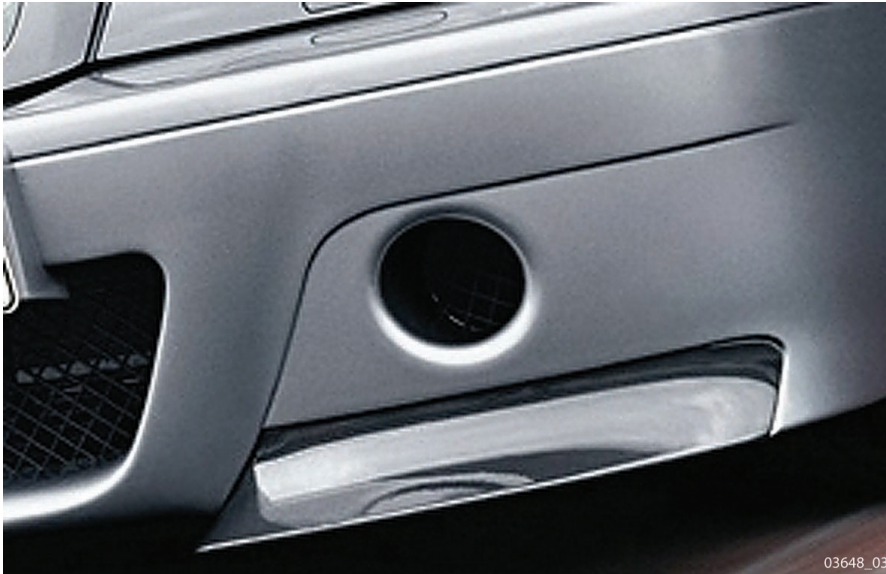
Fig. 18: Air-intake scoop in front valance
