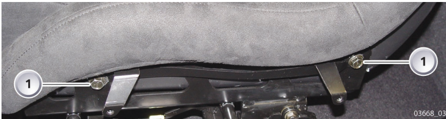
Fig. 13: Bucket-seat fixing bolts (1)
