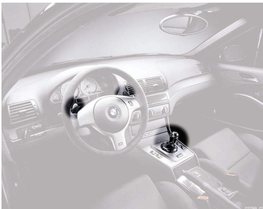
Fig. 29: Gear-shift paddles and SMG gear lever
