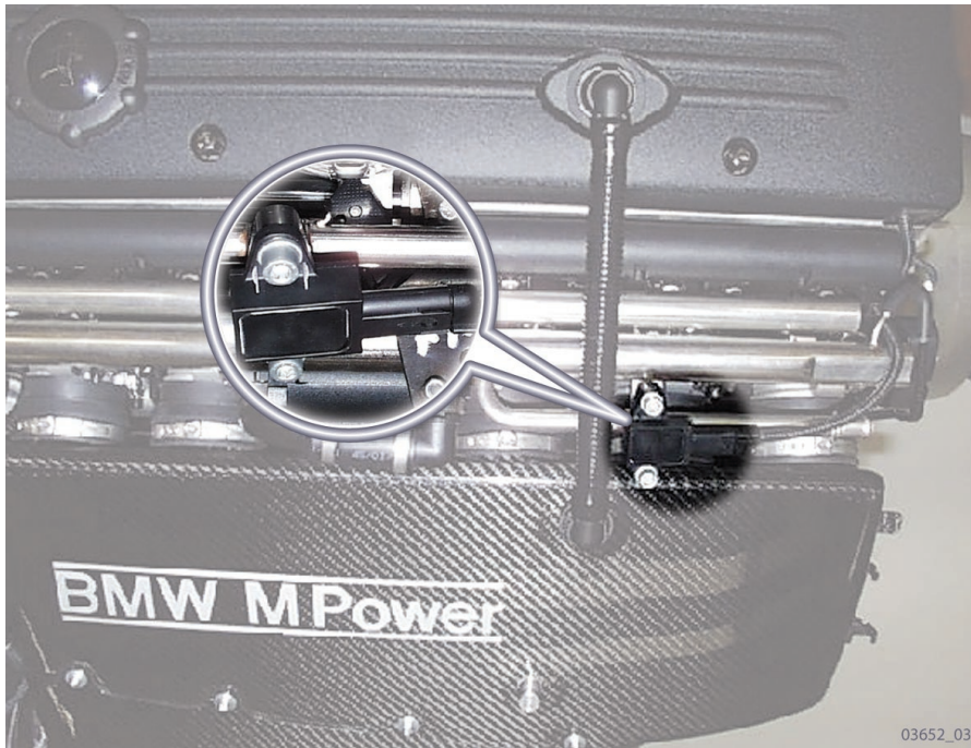
Fig. 23: Pressure sensor on idle-air rail
