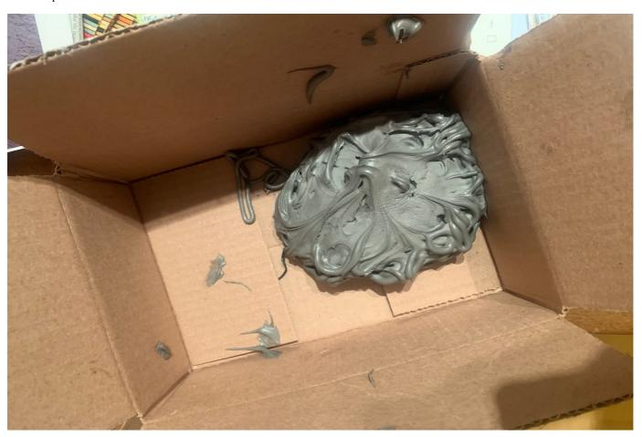
As can be seen, the foam does expand slightly when cured but is not self-leveling. Given this, I think it is pretty important to inject the foam on both sides of each mount since I don't think gravity will evenly distribute the foam. I suspect a lot of it could end up towards the center of the lower cavity if injected only in holes B and D.
