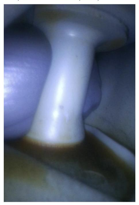
As can be seen, the foam is beginning to surround the mount even before the curing expansion process - which is exactly what you want to see.
