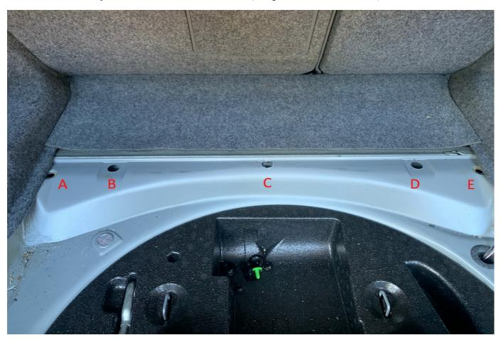
A total of five holes can be seen. Four are existing factory holes (A, B, D, E) and are plugged from the factory. Hole C is user-drilled. A 1cm tall cavity extends the width of the trunk under the area from A to E. A taller cavity containing the mounts sits directly under this. The left rear mount sits in this lower cavity between holes A and B and the right rear mount sits between holes D and E. The five holes have matching holes in the roof of the lower cavity so there is direct access to it.
