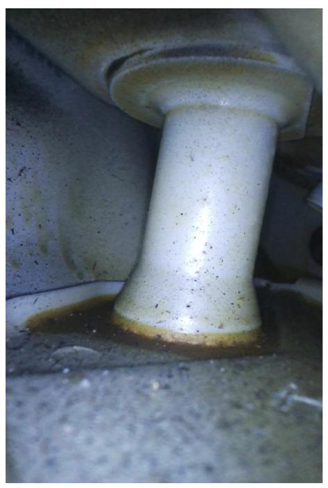
And, finally, here is the right front mount after foam is injected on the opposite side of it.
