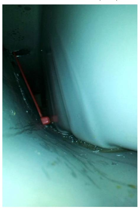
The BMW procedure involves sealing off the left side of the lower cavity from the right by injecting the gap filler into hole C. Here is a view of the area under hole C with the gap filler shown immediately after injection.
