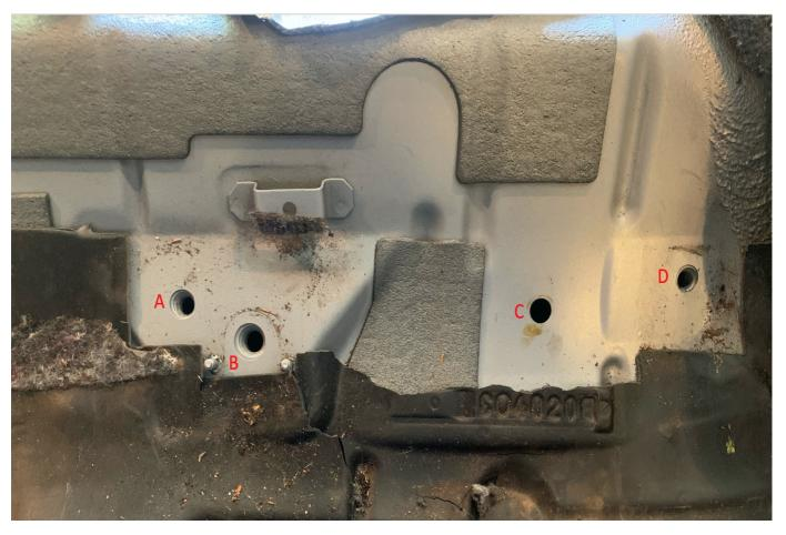
All four holes are factory drilled. Holes A and D are tapped for the rear left seat hinge brackets, B is tapped to hold the rear left seatbelt, and C is unused and has a factory plug.
