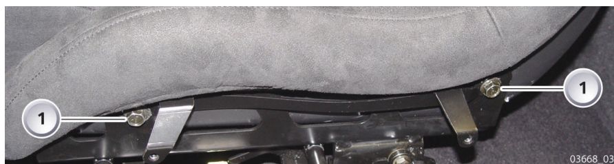
Fig. 13: Bucket-seat fixing bolts (1)
