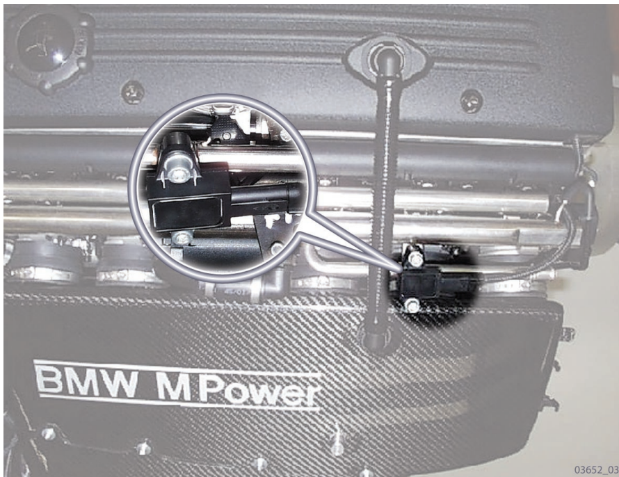
Fig. 23: Pressure sensor on idle-air rail
