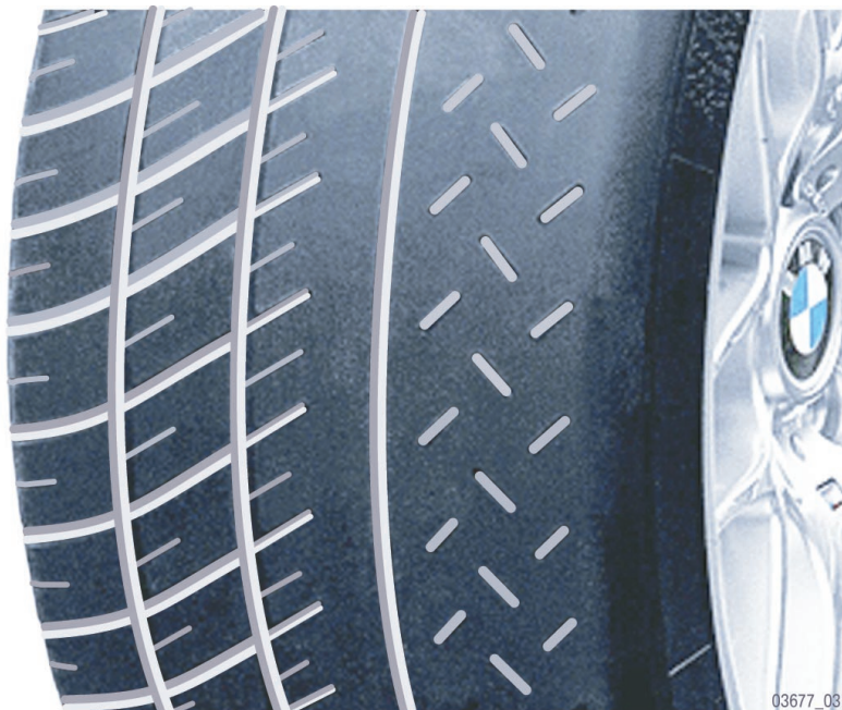
Fig. 32: Tread pattern of Cup tyre
